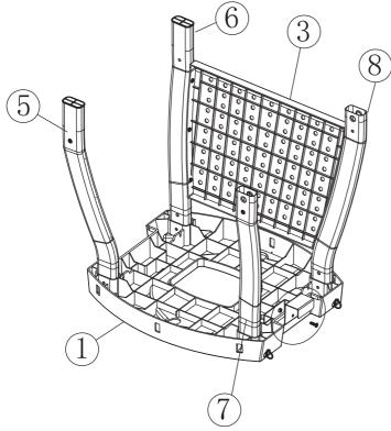
Secure each leg with one M6 x 50mm BOLT (M) and one M6 NUT (N). DO NOT fully tighten yet.
