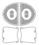
Two shelves are provided and are easily fitted into the corresponding slots located on both sides of the barbeque.
