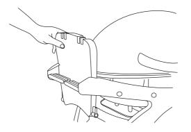
Finally insert the grease tray. Check regularly and replace when necessary.
