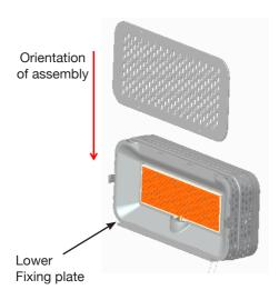
(1) Slide the front panel into the heater from top to bottom. Ensure that it is held in place by the buckles on the left and right sides of the heater. As seen below
