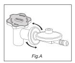
9kg ALVA cylinder recommended with a 5/8" BSP thread; horizontal exit valve. The Bullnose Regulator (not supplied with the heater) tightens to the left hand side (anticlockwise) (figure A).
