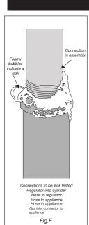
The leak test must be carried out in a well-ventilated area, free from any flames or other sources of ignition.
