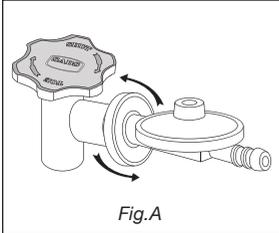
This patio heater makes use of an industrial cylinder (9kg ALVA cylinder recommended) with a 5/8" BSP thread; horizontal exit valve.
