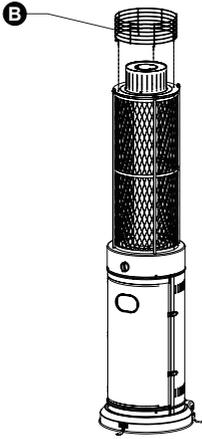
Assemble the upper protective mesh to the heating body directly.
