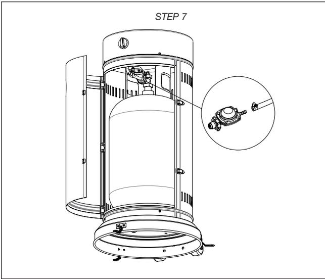
Connect the gas hose and regulator to the heater.
