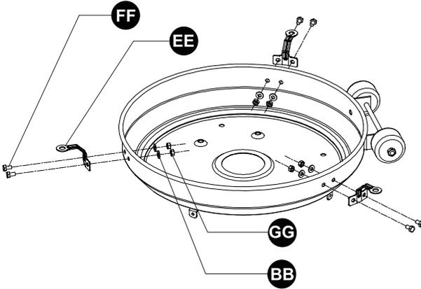
To protect your heater from strong winds, anchor the base securely to the ground with screws. Reverse the base, fix the ground fixer to the base with bolt M6x10 and washer Ø6 like picture shows. Secure the ground fixer with nut M6. Fix another two ground fixer with bolts and nuts, and reverse the base.
