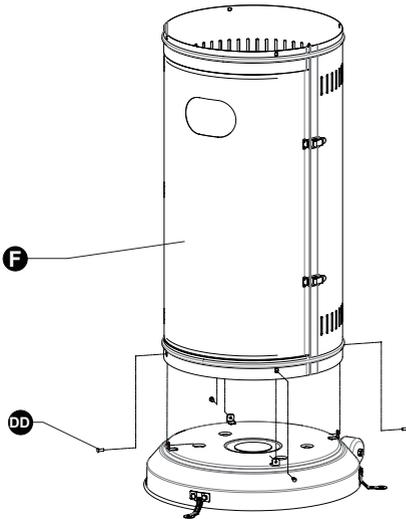
Assemble the tank housing.
