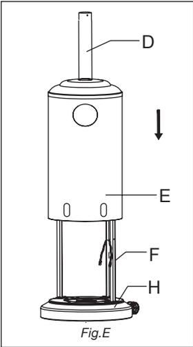
7. Load the Cylinder housing assembly (E) onto the pole (D), and slide the Cylinder Housing Assembly (E) down. (Figure E)
