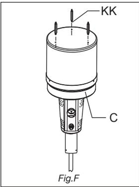
8. Screw Reflector Spacers (KK) into top of Burner Assembly (C).
