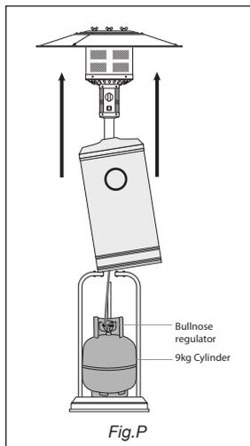
Make sure your cylinder valve is closed (by turning it clockwise). Allow the heater to fully cool before replacing the cylinder. Open the heater to expose the cylinder.
