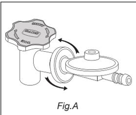
This patio heater makes use of an industrial cylinder (9kg ALVA cylinder recommended) with a 5/8" BSP thread; horizontal exit valve. The Bullnose regulator supplied with the heater tightens to the left hand side (anti-clockwise). (*Figure A*).
