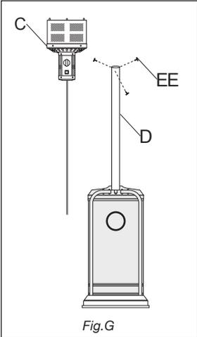
9. Connect the Burner Assembly (C) to the pole (D). Align the screw holes and secure burner assembly (C) onto pole (D) with M5 X 12 pan head bolts (EE). (Figure G)
