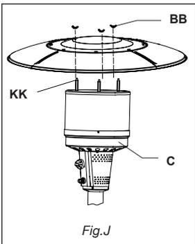
11. Attach dome assembly to burner assembly (C) by securing wing nuts (BB) to reflector spacers (KK). (Figure J)
