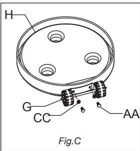
5. Attach wheel assembly (G) to the base (H) using M8 x 15mm bolts (AA) and M8 nuts (CC). (Figure C)
