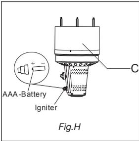
9. a. Open the igniter cap by unscrewing the cap counterclockwise.
