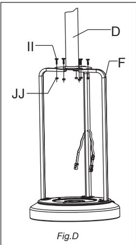
6. Attach pole (D) onto the support brackets (F) using M6 x 25 Hexagon Head Bolts (II) and M6 Nuts (JJ). (Figure D)
