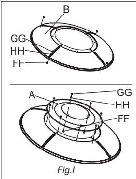
10. Attach KD Domes (B) using M5 x 8mm bolts (FF), M5 Nuts (GG) and 5mm washers (HH). Then, complete dome assembly by attaching top dome (A) to KD dome (B) with M5 x 8mm bolts (FF), M5 Nuts (GG) and 5mm washers (HH). (Figure I)
