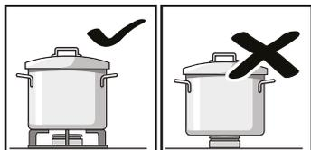
Place the pans on the pan supports, never directly on the burner. Pans should be placed on the hob carefully.
