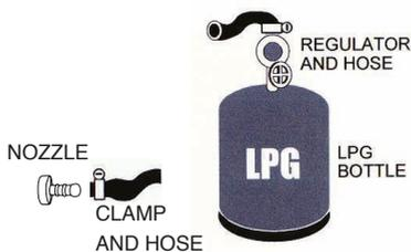
NOTE: After installing and connecting the hose to the hob and regulator, and the regulator to the gas cylinder, a gas leak test must be performed as detailed on page 8 of the booklet.
