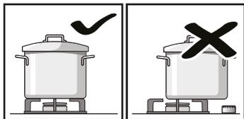
Always centre the pan over the burner, not to one side. Otherwise it could tip over. Do not place large pans on the burners near the control knobs. These may be damaged by the very high temperature.
