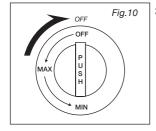
3. Depress the control knob onto the valve spindle. (Fig. 10)
