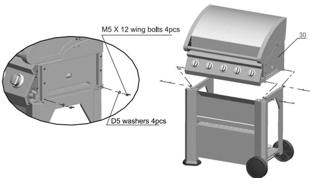
Place the grill body (30) onto the assembled cart, secure with 4pcs D5 washers and 4pcs M5x12 wing bolts.
