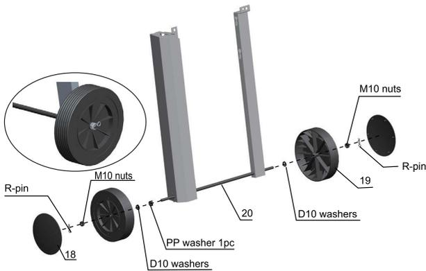
Attach (1) PP washer (GG), (2) D10 washers (EE), (2) wheels (#19), (2) M10 nuts (HH), (2) R-pins (FF) and (2) wheel caps (#18) to the axle (#20) and secure them in turn as above.
