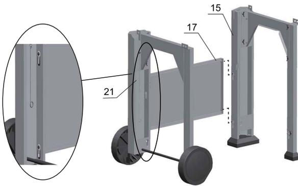
Insert the (4) pre-installed bolts on lower front panel (#17) into the key holes on front left pole (#15) and front right pole (#21), press down to position as illustrated.
