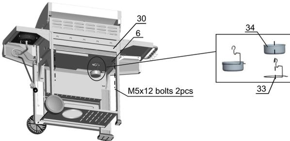
Fix grease tray (6) onto the grill body (3) with 2pcs M5 x 12 bolts, install grease cup (34) into grease cup hanger (33) and then hang them onto the bottom of the grease tray.
