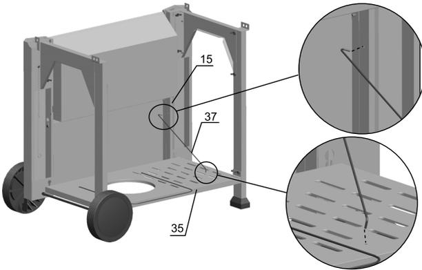
Insert the ends of the connection bar (37) into the holes on the front left pole (15) and the bottom panel (35) as illustrated above.
