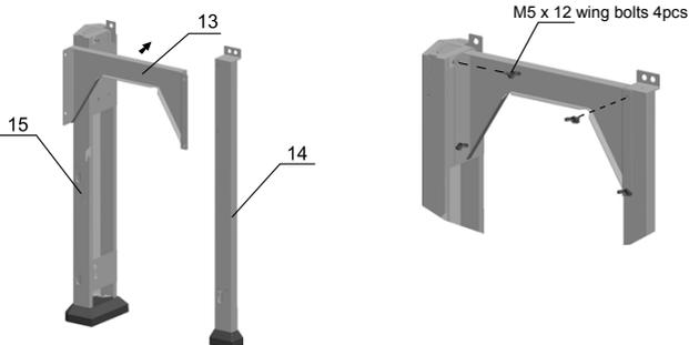
Attach left transom (#13) to front left pole (#15) and rear left pole (#14), fix them with (4) M5 x 12 wing bolts (AA).
