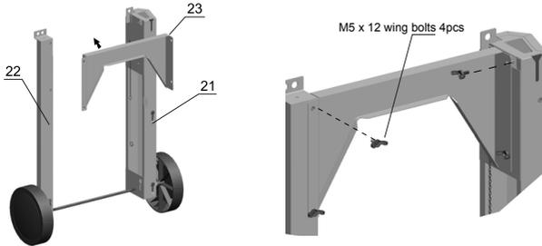
Attach right transom (#23) to front right pole (#21) and rear right pole (#22), fix them with (4) M5 x 12 wing bolts (AA).
