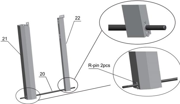
Insert the axle (#20) through the front right pole (#21) and rear right pole (#22), secure them with (2) R-pins (FF).
