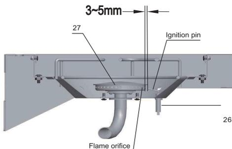
Insert the end of the ignition wire to the ignition pin (26) on the right side burner bowl (25). Note: Manually adjust the gap between the ignition pin and the flame orifice around 3-5mm (0.1-0.2 inch) to ensure proper ignition.
