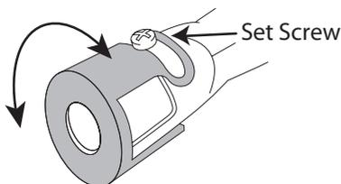
The Side Burner has an adjustable air control should the flame not be correct, i.e.
