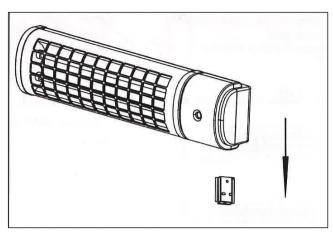
Align the back card slot with the fastening bracket, and fix the product along the direction of the arrow.
