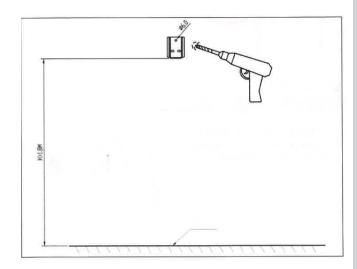
Drill 3 holes with diameter 6mm from the wall, to match the holes in the fastening bracket.
