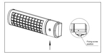
Hang the device on the wall and tighten one ST3.9x12 screw on the bottom to fix the device totally.
