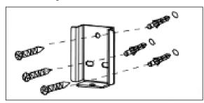
Clean the drill hole from the drilling dust because the wall plugs could otherwise jam, insert the wall plugs into the holes. Firmly screw in the fastening bracket.
