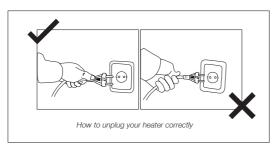
To remove from the socket pull on the plug, not the electrical cord
