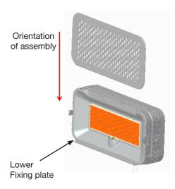
(1) Slide the front panel into the heater from top to bottom. Ensure that it is held in place by the buckles on the left and right sides of the heater. As seen below
