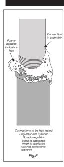
The leak test must be carried out in a well-ventilated area, free from any flames or other sources of ignition.
