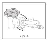
9kg ALVA cylinder recommended with a 5/8" BSP thread; horizontal exit valve. The Bullnose Regulator tightens to the left hand side (anticlockwise) (Fig. A).
