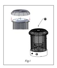
Insert the upper safety guard 4pcs feet into the lower guard 4pcs holes shown in (Figure I), the upper safety guard middle hole on the reflector stud.
