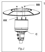
Attach dome assembly to burner assembly (C) by securing wing nuts (BB) to reflector spacers (KK). (Figure J) (BB) Wing Nut
