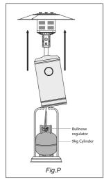
Make sure you cylinder valve is closed (by turning it clockwise). Allow the heater to fully cool before replacing the cylinder. Open the heater to expose the cylinder. Lift up the tank housing and tilt it so that the tank housing support holds the cylinder housing up, exposing the cylinder fully, allowing you to access and replace the cylinder. When replacing the cylinder secure in position with strap. (*Figure P*)
