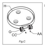
Attach wheel assembly (G) to the base (H) using M8 x 15mm bolts (AA) and M8 nuts (CC). (Figure C)
