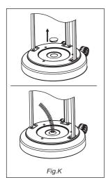
Open the base cap, fill up the weight box using 12kgs of sand or soil, and the lock the weight based cap back. (*Figure K*)
