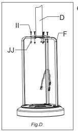
Attach pole (D) onto the support brackets (F) using M6 x 25 Hexagon Head Bolts (II) and M6 Nuts (JJ). (Figure D)
