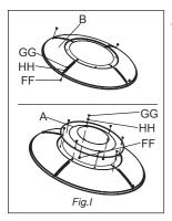
Attach KD Domes (B) using M5 x 8mm bolts (FF), M5 Nuts (GG) and 5mm washers (HH). Then, complete dome assembly by attaching top dome (A) to KD dome (B) with M5 x 8mm bolts (FF), M5 Nuts (GG) and 5mm washers (HH). (*Figure I*)
