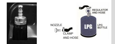
NOTE: After installing and connecting the hose to the hob and regulator, and the regulator to the gas cylinder, a gas leak test must be performed as detailed on page 8 of the booklet.
