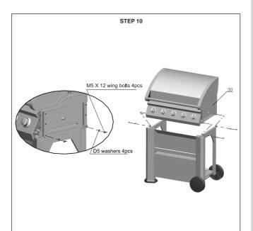
Place the grill body (30) onto the assembled cart, secure with 4pcs D5
