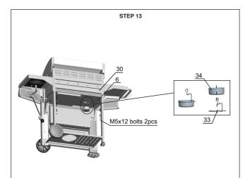
Fix grease tray (6) onto the grill body (3) with 2pcs M5 x 12 bolts, install grease cup (34) into grease cup hanger (33) and then hang them onto the bottom of the grease tray.
