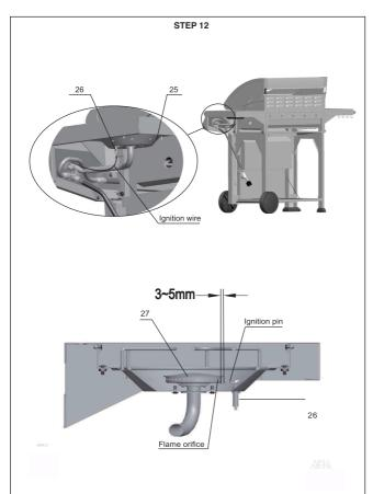
Insert the end of the ignition wire to the ignition pin (26) on the right side burner bowl (25). Note: Manually adjust the gap between the ignition pin and the flame orifice around 3-5mm (0.1-0.2 inch) to ensure proper ignition.
