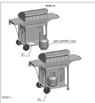
Place the gas cylinder (not included) into the hole at the bottom panel (21) Left the cylinder fixing hook (31) to secure the gas cylinder
