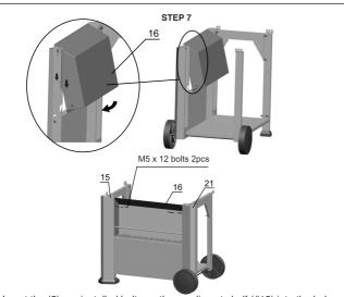
Insert the (2) pre-installed bolts on the condiment shelf (#16) into the holes on top of the front left pole (#15) and front right pole (#21), slide down and then place another (2) pre-installed bolts on the condiment shelf (#16) to position shown above.
