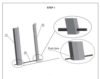
Insert the axle (#20) through the front right pole (#21) and rear right pole (#22), secure them with (2) R-pins (FF).
