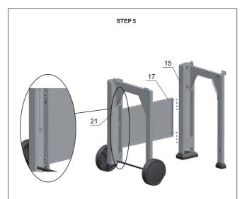
Insert the (4) pre-installed bolts on lower front panel (#17) into the key holes on front left pole (#15) and front right pole (#21), press down to position as illustrated.
