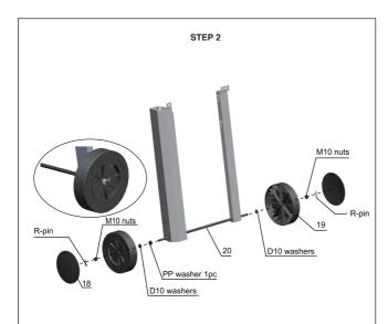
Attach (1) PP washer (GG), (2) D10 washers (EE), (2) wheels (#19), (2) M10 nuts (HH), (2) R-pins (FF) and (2) wheel caps (#18) to the axle (#20) and secure them in turn as above.
