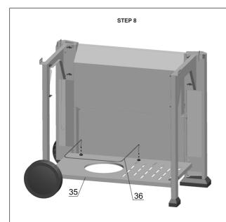
Insert the cylinder fixing hook (36) into the two holes on the bottom panel (35)
