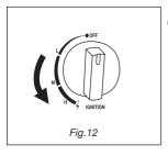
You can now turn on the unit. Turn the control knob anti-clockwise until you hear a 'Click'. Repeat if necessary after waiting 20 seconds. (Fig.12)
