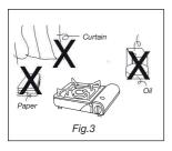
Make sure that there are no flammable materials near the gas cooker. (Fig. 3)
