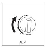
After use, turn the ignition knob to the OFF position "OFF", and make sure the burners are OFF. (Fig. 4)
