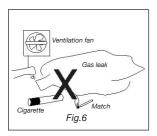
When detecting a gas leak or if you smell gas, perform a Leak test (*Page.6*). DO NOT test for a leak using an open flame or ignition source.
