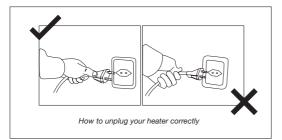
To remove from the socket pull on the plug, not the electrical cord
